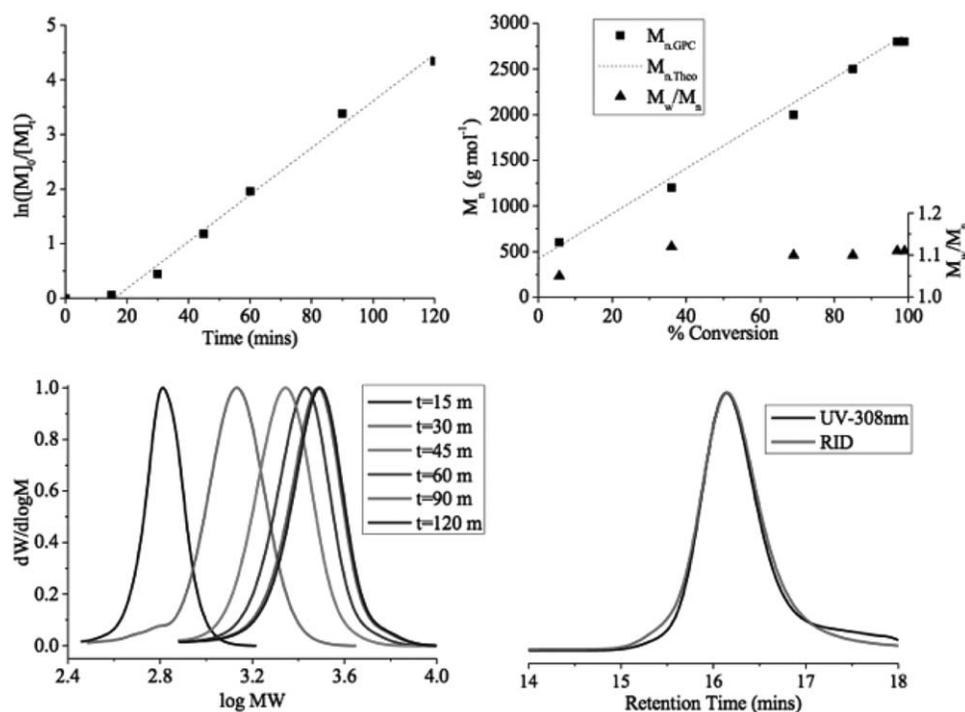
**FIGURE 3** Characterization for the RAFT homopolymerization of DMA. Semi logarithmic plot (*top left*), measured and theoretical  $M_n$  of P(DMA) against total monomer conversion (*top right*), evolution of GPC traces of P(DMA) over time (*bottom left*), VWD (308 nm) and RID GPC traces of sample P1 after precipitation (*bottom right*). [Color figure can be viewed in the online issue, which is available at [wileyonlinelibrary.com](http://wileyonlinelibrary.com).]
