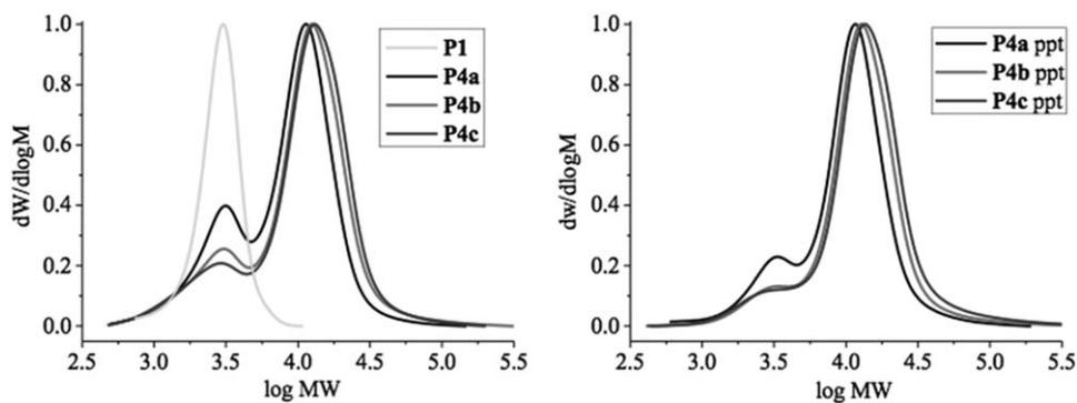
**FIGURE 6** GPC traces of P(DMA) and crude P[(DMA)-*b*-(PIBA)]s (*left*) and GPC traces of precipitated P[(DMA)-*b*-(PIBA)]s (P4a-c) (*right*). [Color figure can be viewed in the online issue, which is available at [wileyonlinelibrary.com](http://wileyonlinelibrary.com).]
