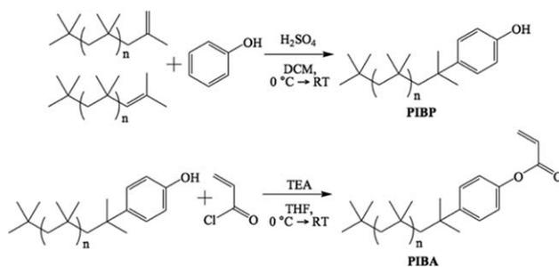
**SCHEME 1** Synthesis of PIBP by Friedel-Crafts alkylation of phenol with vinylidene/trisubstituted olefin PIB (*top*), synthesis of PIBA by esterification of PIBP with acryloyl chloride (*bottom*).
