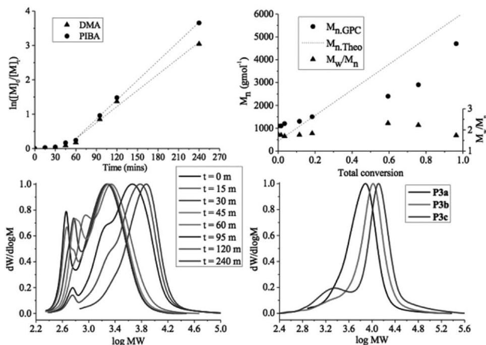
**FIGURE 5** Characterization for the RAFT copolymerization of DMA and PIBA; semi logarithmic plot (*top left*), measured and theoretical  $M_n$  of P[(DMA)-*co*-(PIBA)] against total monomer conversion (*top right*), evolution of GPC traces of P[(DMA)-*co*-(PIBA)] over time (*bottom left*), GPC traces of P[(DMA)-*co*-(PIBA)] samples P3a-c (*bottom right*). [Color figure can be viewed in the online issue, which is available at [wileyonlinelibrary.com](http://wileyonlinelibrary.com).]
