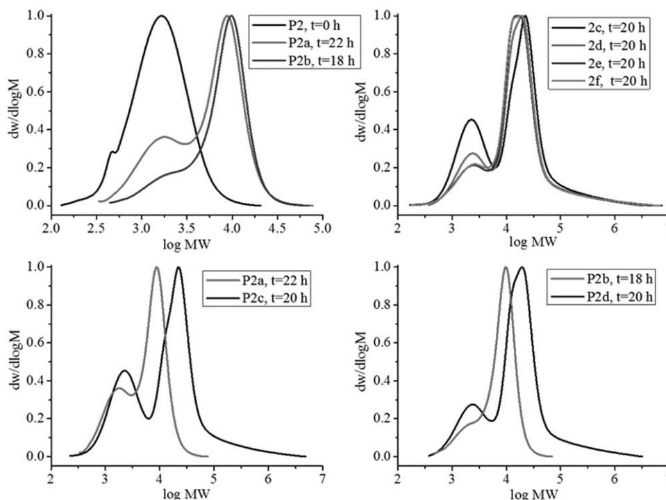
**FIGURE 4** GPC traces of P(PIBA) (P2a/b) synthesized by RAFT polymerization (*top left*) GPC traces of P(PIBA) (P2c-f) synthesized by free radical polymerization (*top right*) GPC traces of P(PIBA) synthesized with 0.1 (*bottom left*) or 0.25 (*bottom right*) equivalent of V601 with and without RAFT agent present. [Color figure can be viewed in the online issue, which is available at [wileyonlinelibrary.com](http://wileyonlinelibrary.com).]
