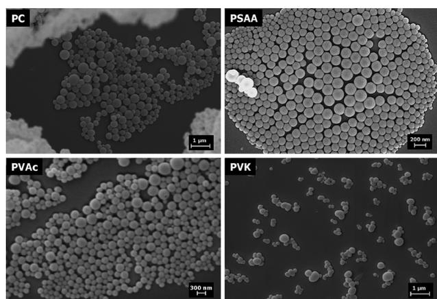
**Fig. 1** SEM images of polymeric nanoparticles of poly(carbonate) (PC), poly(styrene-*co*-acrylic acid) (PS-*co*-AA), poly(vinyl acetate) (PVAc) and poly(vinyl carbazole) (PVK) prepared by dialysis of the polymers.
