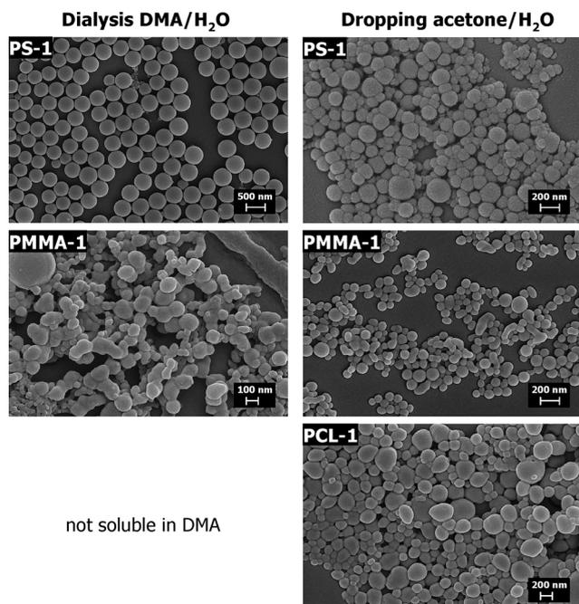
**Fig. 2** SEM images of polymeric nanoparticles of poly(styrene) (PS), poly(methyl methacrylate) (PMMA), poly( $\epsilon$ -caprolactone) (PCL) prepared by dialysis of the polymers dissolved in DMA ( $c = 4$  mg/mL) and by dropwise addition of water into an acetone solution of the polymers containing 4 mg/mL.
