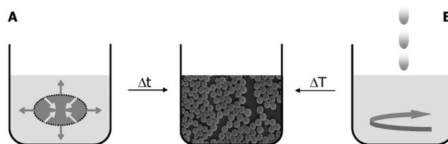
**Scheme 1** A schematic representation of the nanoprecipitation methods applying dialysis in a membrane (A) and the dropping technique under stirring (B), respectively.
