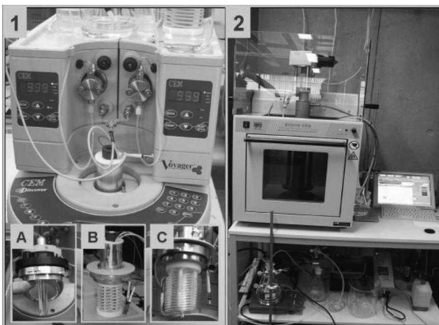
**Figure 1.** Pictures of the utilized microwave synthesizers: CEM Voyager™ equipped with a 10 mL tube reactor (system 1A), 5 mL Teflon coil (system 1B), or 10 mL glass coil (system 1C) and the Milestone FlowSYNTH equipped with a 200 mL CSTR (system 2).
